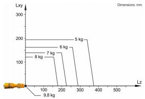
The KR 8 R2010-2 is designed for a rated payload of 8 kg in order to optimize the dynamic performance of the robot. The maximum payload of 9.8 kg applies only if the position of the center of mass is 0 mm and a supplementary load optimized for the load case is mounted. The specific load case must be verified using KUKA.Load or KUKA Compose. For further consultation, please contact KUKA Support.
