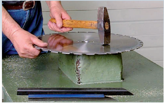
Feinrichten · High-precision straightening of the blades
