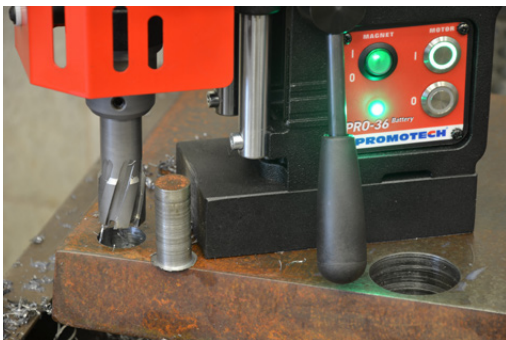
Milling capacity up to 36 mm (1 7/16") • Max depth of cut up to 50 mm (1.97")
