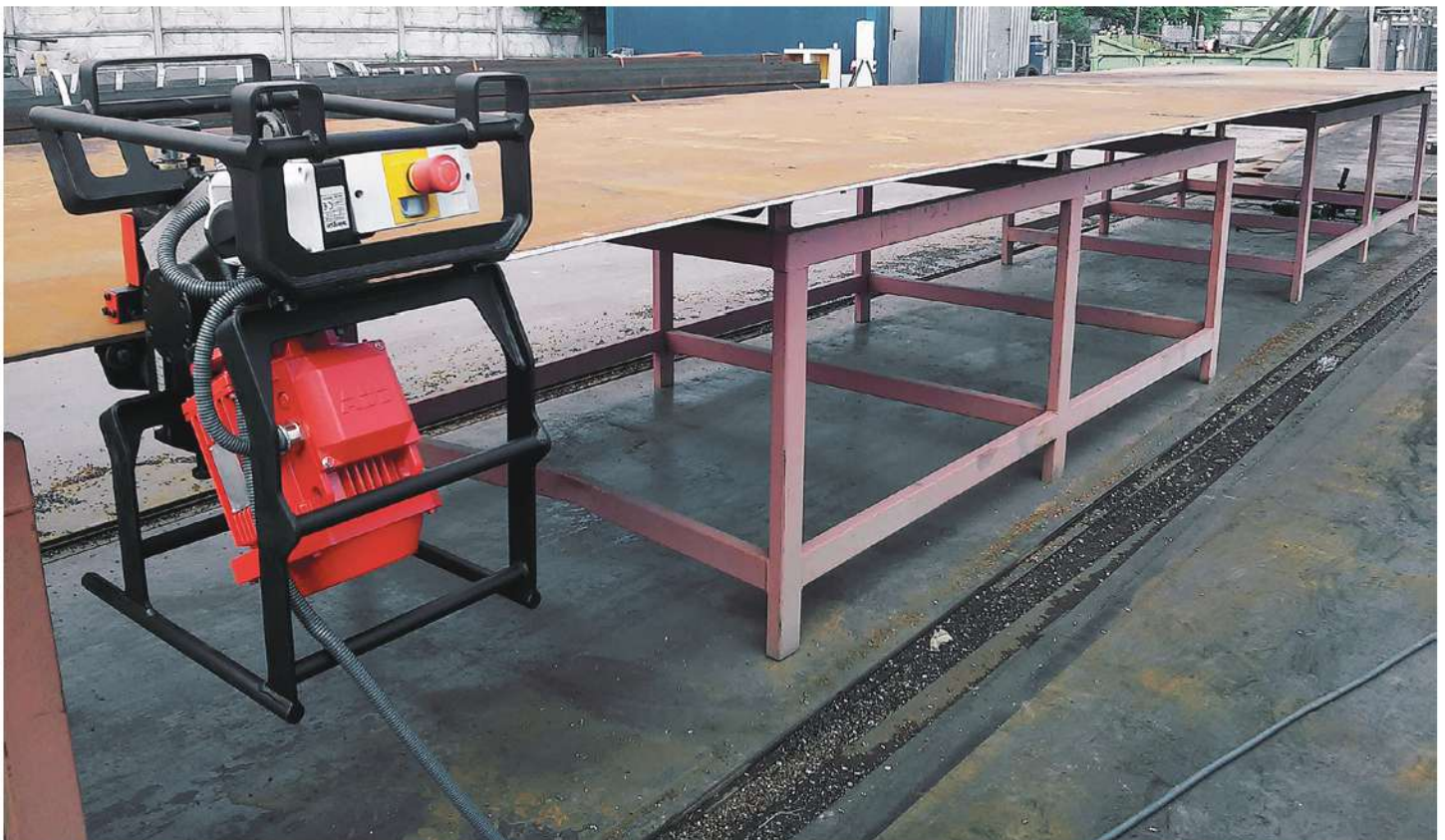
ABM-14 runs along a plate automatically
