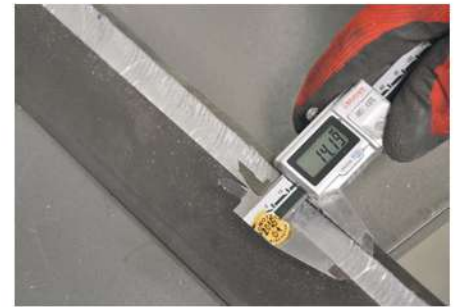
Maximum bevel width up to 14 mm
