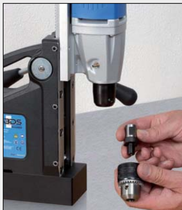
1. Connect adapter to drill chuck.
