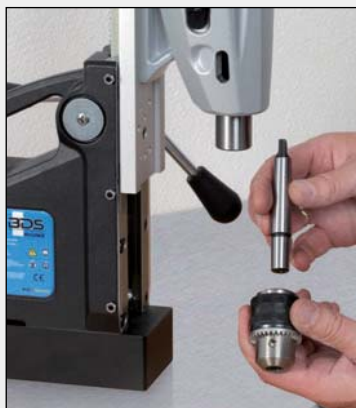
1. Connect taper drift to drill chuck.
