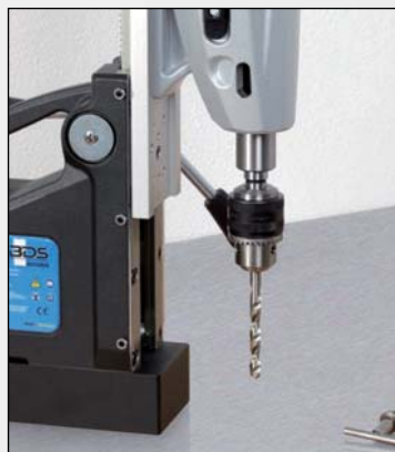
3. Ready for use with twist drill.
