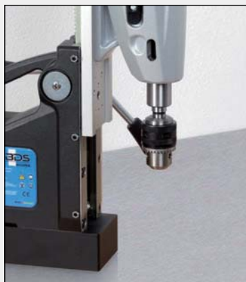
2. Place drill chuck in MT arbor.
