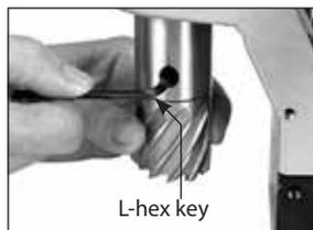
**CAUTION:** Ensure that the locking screw is on a flat of the cutter and not just against the rounded shank.
