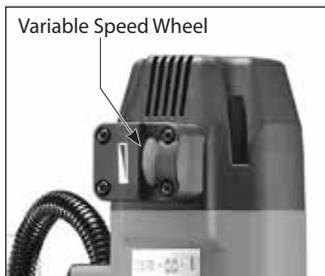
**Avoid overheating the motor:** When using the machine at or near maximum capacity with a slow motor speed the motor will be at maximum stress and very hot. After each cut is finished, ALWAYS cool the motor by running at no load at the maximum motor speed for a few minutes.
