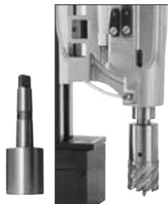
**WARNING: Do not use larger than 60mm cutters in a quick release arbor.**
