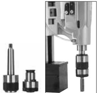
Allow the machine to come to a full stop. Then reverse direction and restart machine by pressing the green motor switch to remove tap. Guide the tap back out with the feed handle. Proper order of operations for normal tapping is as follows: magnet: on. direction: forward. motor: on. motor: off. THEN: direction: reverse. motor: on. motor: off - magnet: off.
