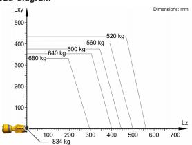
The KR 640 R2800-2 is designed for a rated payload of 640 kg in order to optimize the dynamic performance of the robot. With reduced load center distances and favorable supplementary loads, a maximum payload of up to 834 kg can be mounted. The specific KUKA Load case must be verified using KUKA. For further consultation, please contact KUKA Service.
