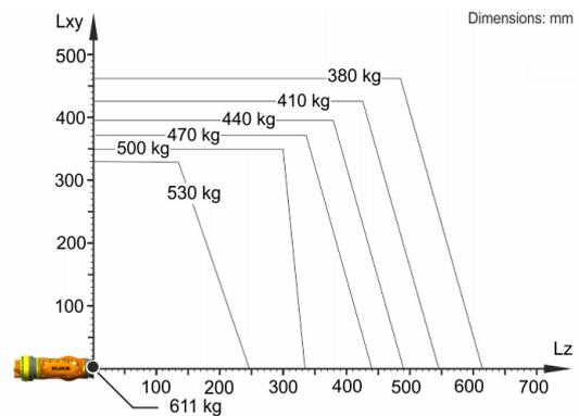
The KR 500 R2830 MT-F is designed for a rated payload of 500 kg in order to optimize the dynamic performance of the robot. The maximum payload of 611 kg applies only if the position of the center of mass is 0 mm and a supplementary load optimized for the load case is mounted. The specific load case must be verified using KUKA.Load or KUKA Compose. For further consultation, please contact KUKA Support.
