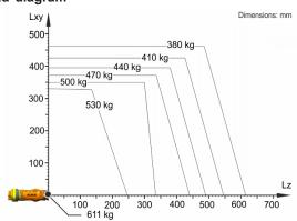
The KR 500 R2830 C is designed for a rated payload of 500 kg in order to optimize the dynamic performance of the robot. The maximum payload of 611 kg applies only if the position of the center of mass is 0 mm and a supplementary load optimized for the load case is mounted. The specific load case must be verified using KUKA.Load or KUKA Compose. For further consultation, please contact KUKA Support.
