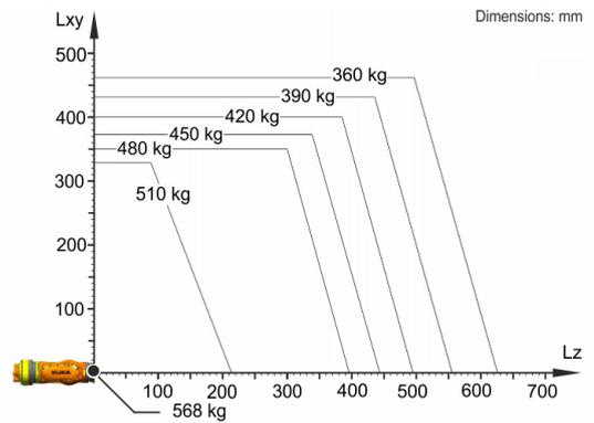
The KR 480 R3330 MT is designed for a rated payload of 480 kg in order to optimize the dynamic performance of the robot. The maximum payload of 568 kg applies only if the position of the center of mass is 0 mm and a supplementary load optimized for the load case is mounted. The specific load case must be verified using KUKA.Load or KUKA Compose. For further consultation, please contact KUKA Support.
