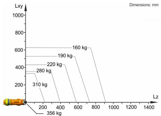
The KR 280 R3080 F is designed for a rated payload of 280 kg in order to optimize the dynamic performance of the robot. The maximum payload of 356 kg applies only if the position of the center of mass is 0 mm and a supplementary load optimized for the load case is mounted. The specific load case must be verified using KUKA.Load or KUKA Compose. For further consultation, please contact KUKA Support.
