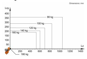
The KR 140 R3200-2 PA is designed for a rated payload of 140 kg in order to optimize the dynamic performance of the robot. With reduced load center distances and favorable supplementary loads, a maximum payload of up to 180 kg can be mounted. The specific KUKA Load case must be verified using KUKA. For further consultation, please contact KUKA Service.
