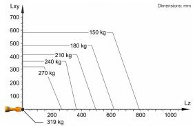
The KR 240 R2900-2 is designed for a rated payload of 240 kg in order to optimize the dynamic performance of the robot. The maximum payload of 319 kg applies only if the position of the center of mass is 0 mm and a supplementary load optimized for the load case is mounted. The specific load case must be verified using KUKA.Load or KUKA Compose. For further consultation, please contact KUKA Support.
