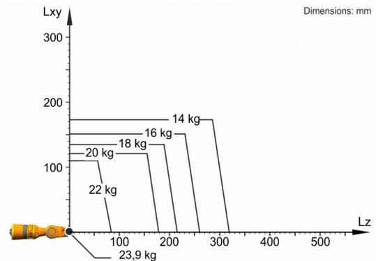
The KR 20 R1810-2 is designed for a rated payload of 20 kg in order to optimize the dynamic performance of the robot. The maximum payload of 23.9 kg applies only if the position of the center of mass is 0 mm and a supplementary load optimized for the load case is mounted. The specific load case must be verified using KUKA.Load or KUKA Compose. For further consultation, please contact KUKA Support.
