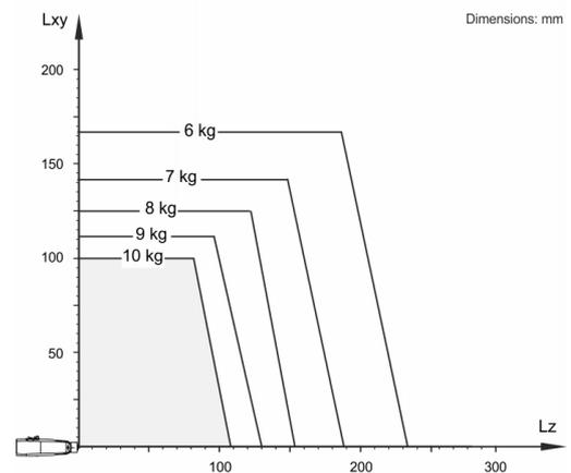
The KR 10 R900 WP is designed for a rated payload of 5 kg in order to optimize the dynamic performance of the robot. The maximum payload of 10 kg applies only if the position of the center of mass is 0 mm and a supplementary load optimized for the load case is mounted. The specific load case must be verified using KUKA.Load or KUKA Compose. For further consultation, please contact KUKA Support.
