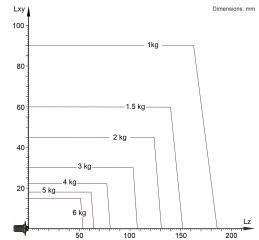
The KR 3 D1200 is designed for a rated payload of 3 kg in order to optimize the dynamic performance of the robot. With reduced load center distances and favorable supplementary loads, a maximum payload of up to 6 kg can be mounted. The specific KUKA Load case must be verified using KUKA. For further consultation, please contact KUKA Service.
